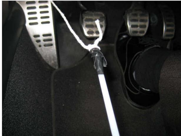
Detach the string from the cable-tie and tie to the 9-pin D connector of the OBD cable. Next, gently start to pull the string back through the air vent opening, pulling the OBD cable back up with it. The cable will snag on the way, each time it snags, pull the OBD cable back down a few centimetres and gently rotate the OBD cable. Eventually the 9-pin D connector will emerge from the air vent opening.
