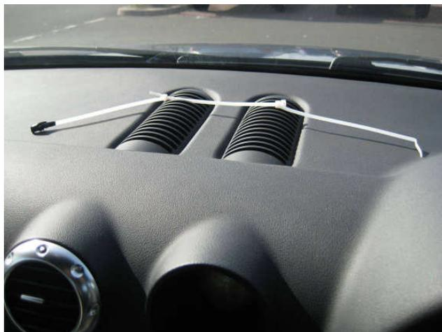
Next feed the cable ties into the dash air vent opening on the right side in a downwards and right direction towards the back of the driver's foot well area.
