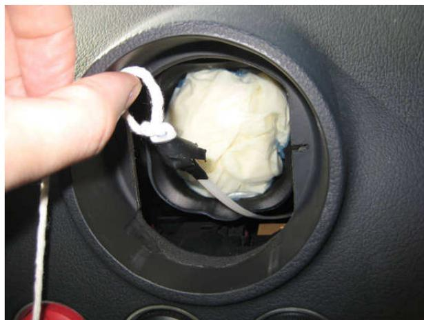
Pull on the bottom of the cable tie until the string emerges in the footwell.
