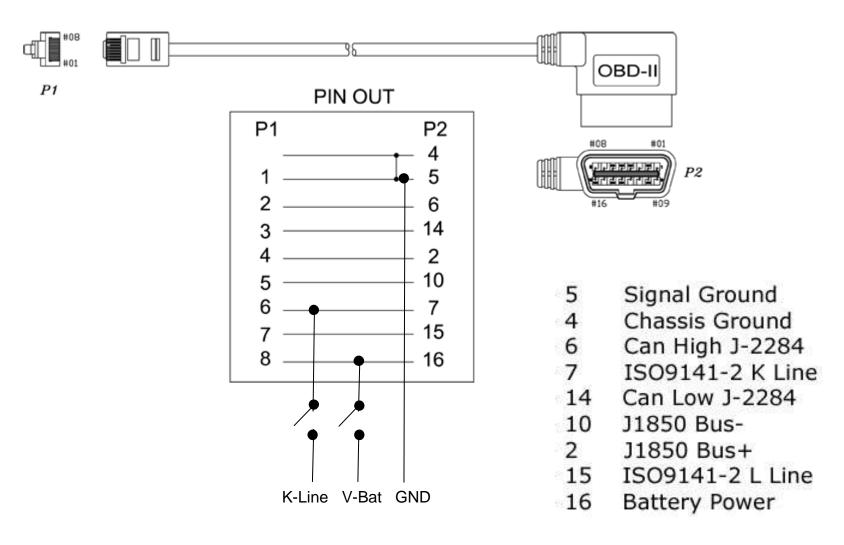
It is recommended to include an in line switch so that the unit can be isolated when connected to a workshop diagnostic tester.
