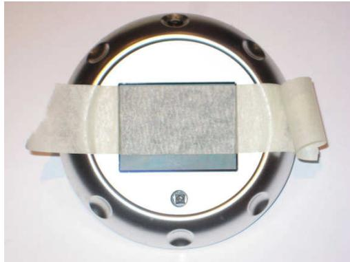
Next glue the PCB to the air vent control wheel as shown below. Once again match the glue position to that shown in the picture below..
