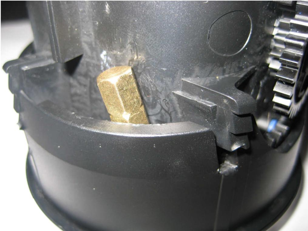
**An alternative and much faster and simpler way is simply to break off the lugs with pliers.**
